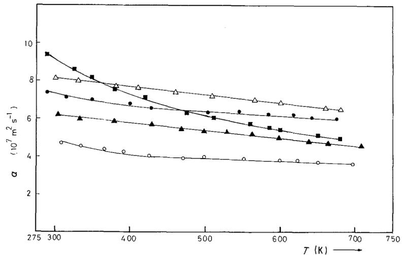
Figure 4 The variation of thermal diffusivity of glass system 77%  $B_2O_3$ -23% PbO doped with ZnO. 0 (■), 1 (△), 2 (●), 3 (▲) and 4 (○) wt %.
