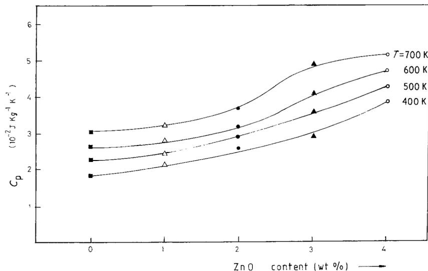
Figure 2 The variation of specific heat capacity with the percentage of ZnO. 0 (■), 1 (△), 2 (●), 3 (▲) and 4 (○) wt %.
