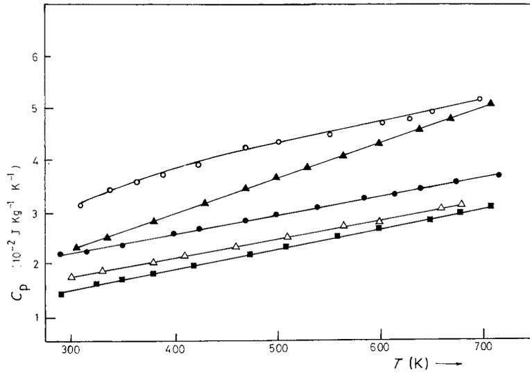
Figure 1 The variation of specific heat capacity with temperature for the glass system 77% B<sub>2</sub>O<sub>3</sub>-23% PbO doped with ZnO at 0 (■), 1 (△), 2 (●), 3 (▲) and 4 (○) wt %.
