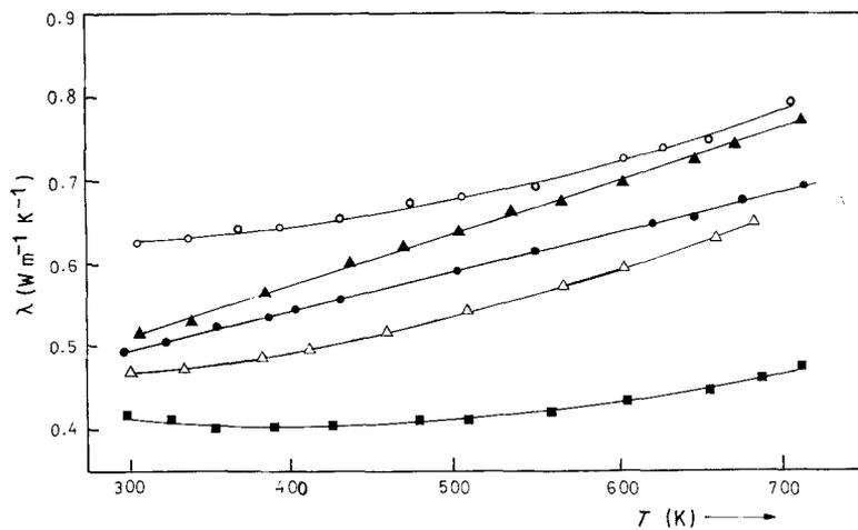
Figure 3 The variation of thermal conductivity for the system 77%  $B_2O_3$ -23% PbO doped with ZnO. 0 (■), 1 (△), 2 (●), 3 (▲) and 4 (○) wt %.
